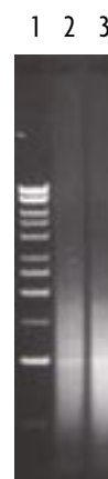
Figure 3: Pure mRNA from total RNA in one passage. mRNA was isolated from 500 µg of total RNA in duplicate, quantified by spectrophotometry and run on a 0.8% agarose gel.
